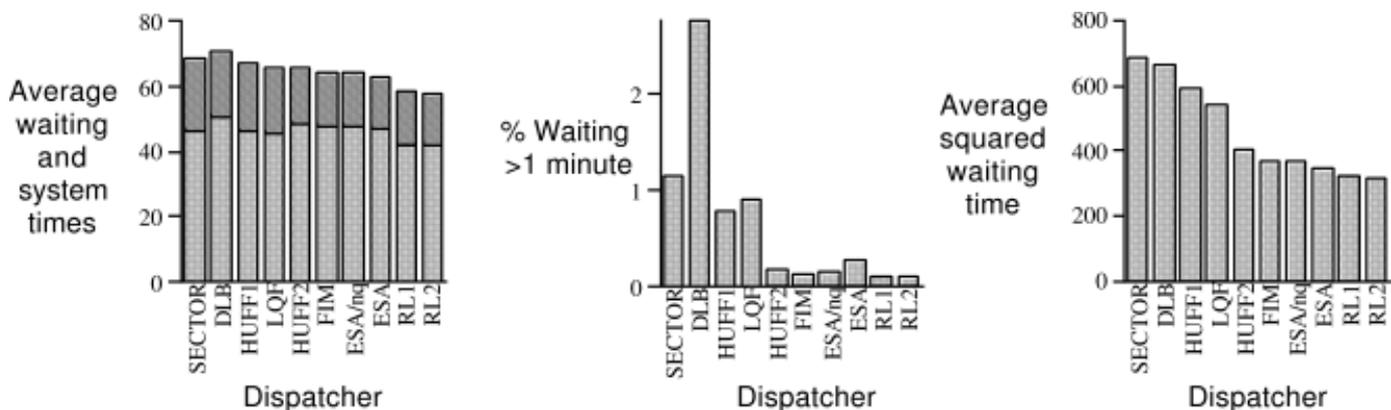
**Figure 11.9:** Comparison of elevator dispatchers. The SECTOR dispatcher is similar to what is used in many actual elevator systems. The RL1 and RL2 dispatchers were constructed through reinforcement learning.
