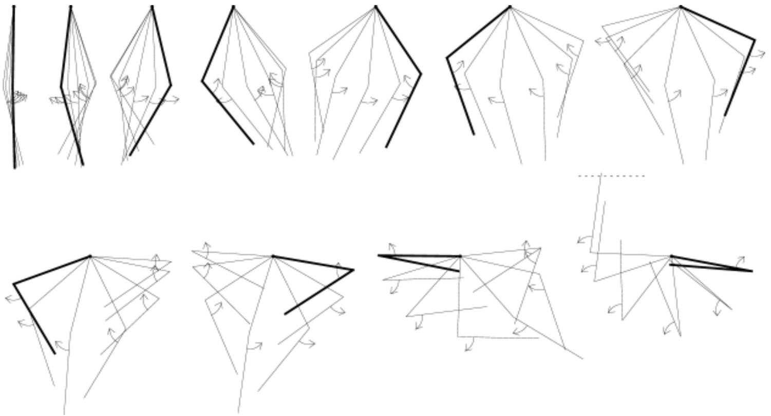
**Figure 11.7:** A typical learned behavior of the acrobot. Each group is a series of consecutive positions, the thicker line being the first. The arrow indicates the torque applied at the second joint.
