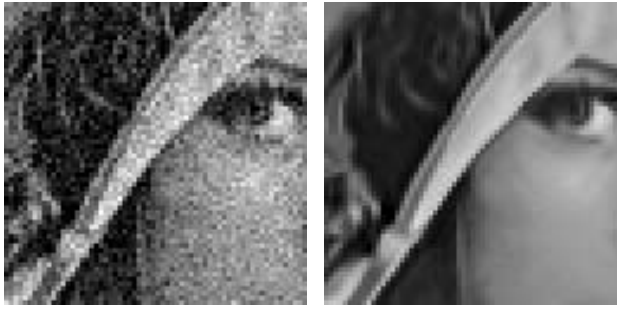
FIG. 9. NL-means denoising experiment with a natural image. Left: Noisy image with standard deviation 20. Right: Restored image.
